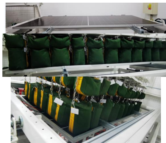
Fig. 10: detail view of mechanical load mounting
