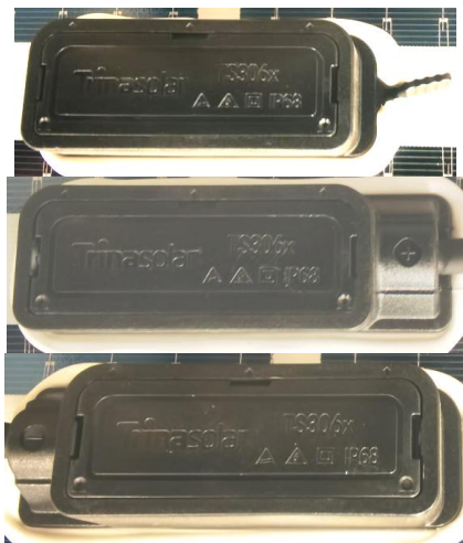
Fig. 15: detail view of closed junction box
